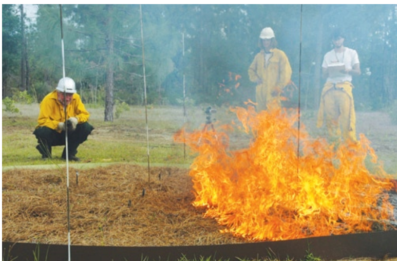
Forest Service and University of Florida researchers carefully monitor the rate of fire spread and other factors through four different mulch types.
